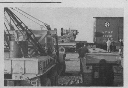
WINCHES GRIND as a 56,000 pound lathe is maneuvered from a flatcar onto a trailer truck. Men of the Shipping and Receiving Division's handling section stand well clear of the straining cables.
